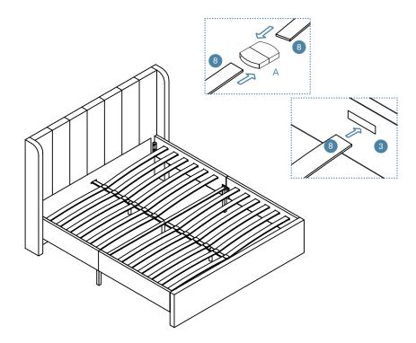
Join the bed planks together in the middle of the frame using 12x double caps (A). Insert the end of the planks into the bed frame as shown and attach the double caps (A) into panel [4]. Make sure the double caps (A) click securely into place.
