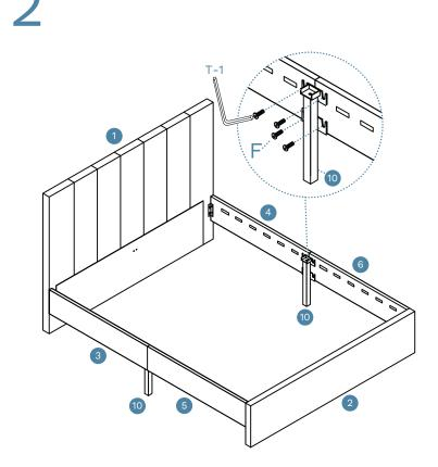
Attach 2 x panels (10) to assembled frame as shown and secure with 8 x bolts (F). Tighten with an Allen Key (T-1).
